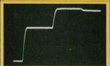
USING EQUIPMENT you already have, you can pinpoint the location of faults along coaxial transmission cables. This technique is especially useful for buried cables. For the complete story, turn to page 67.
