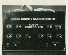
FIG. 38—COMMAND CONSOLE provides the means for controlling remotely via cable.
