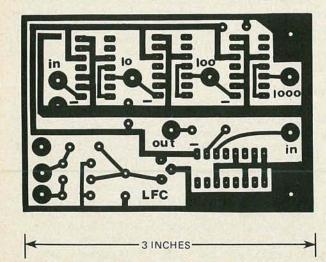
FIG. 3—FOIL PATTERN for the printed-circuit board. Circuit is so simple that using stripboard or perforated board and point-to-point wiring will be a cinch.
