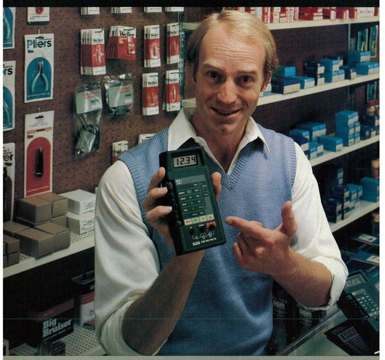
D 804: A powerful, versatile handheld DMM with nine functions, 26 ranges, 0.1% basic dc accuracy and more. Direct temperature readings in °C with K-type thermocouples; peak hold on voltage and current functions; even an audible indicator for instant continuity and logic level detection. Available January 1981. \$229.\*
