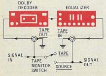
FIG. 2—A DECODER of any sort should always be placed ahead of the equalizer.
