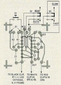
FIG. 3—PARTS PLACEMENT DIAGRAM also indicates connections to components mounted on- and off-board.
