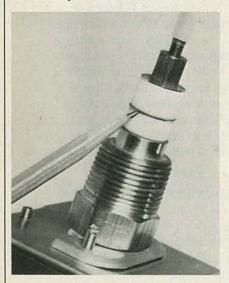
THE GUARD-RING midway down the insulator is connected to the electric line and to the input of the relay coil that holds the circuit closed. When the insulator is clean, it has no effect. If conductive contamination builds up on the insulator, it shunts current around the relay to cause it to drop out, stopping the burner.
