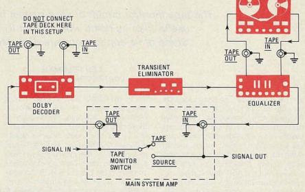
FIG. 4—MANY ADD-ON DEVICES include their own TAPE-IN and TAPE-OUT jacks. Recorder should use jacks on equalizer to take best advantage of its capabilities.
