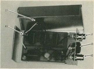
INSIDE VIEW of the low-frequency converter for use with the synthesized function generator and other similar generators. You may want to place the power connector on the end away from the coax connectors.
