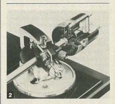
As we mentioned earlier, the combination of a low-mass pickup arm and an ultra-low weight cartridge adds up to a higher natural resonance point that lies above the region of maximum warp-frequency typically found on records—above 8 Hz and below 12 Hz. However, merely moving up the frequency of resonance does not in itself necessarily reduce the amplitude of that resonance.
