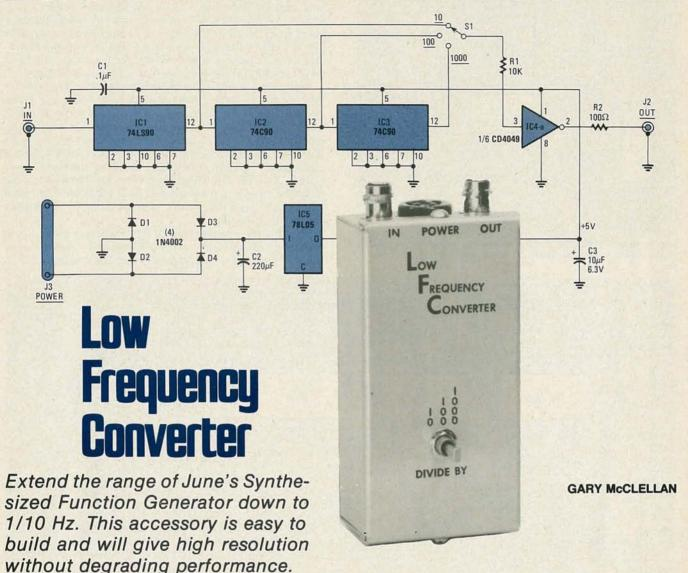
THE CONSTRUCTION ARTICLE ON THE SFG (SYNTHESIZED FUNCton Generator) in the June 1980 issue has caused quite a bit of interest in high-performance function generators. But one of the shortcomings of the SFG project is that it won't go below 100 Hz. That is because of the basic design of that instrument. Any changes in circuitry would increase the time it takes to lock on frequency and its performance would be seriously degraded.
