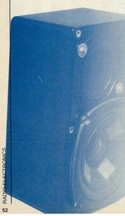
paper material for the cone. It is interesting to note that, although there is nothing in loudspeaker-design theory that dictates that a given driver must have low moving-mass in order to achieve extended high frequency response, in practice it usually works out that way: Heavy cones and moving assemblies usually decouple from the voice coil at high frequencies and simply stop moving.
