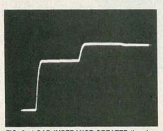
FIG. 3—LOAD IMPEDANCE GREATER than input impedance. Reflected pulse is added to incident pulse.
