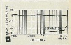
Frequency response of the ULM cartridge is plotted from 20 Hz to 20 kHz (the available frequencies on our test record) in Fig. 5. To obtain that response, we had to add about 200
