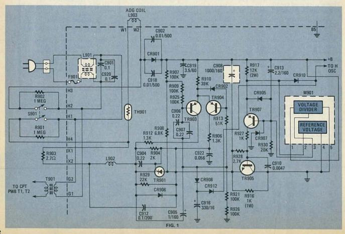
The base voltage of TR907 comes from a voltage-divider/reference-voltage module, which is M901. A tap on the voltage divider develops the base voltage. No resistance values are given for that in the parts lists. It's a ceramic, flat 5-pin device, Hitachi 2370141.
