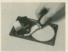
FIG. 6—SILICONE SEALANT holds crossover network components to front panel.
