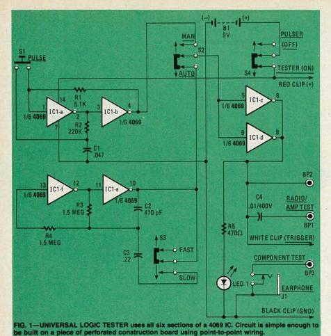
voltage capacitor to protect the IC when testing tube-type audio amplifiers and radios, or when dealing with voltages above 15 volts. The capacitor passes the squarewave pulses, but blocks DC.
