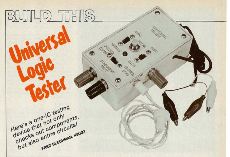
THE UNIVERSAL TESTER IS USED TO troubleshoot digital logic and counting circuits. It performs useful checks of resistors, capacitors, transistors, and most other electronic components. It can also be used to test audio and AM radio circuits.
